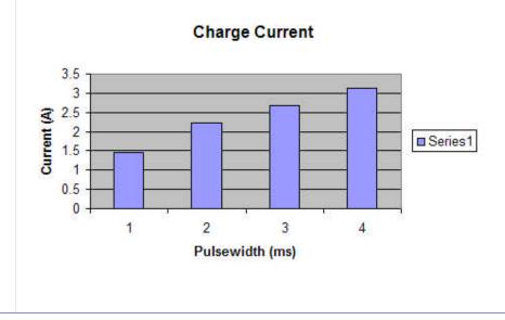
We know what went into the coil pack, now lets look at what comes out. The next measure output current from the LS1 coil pack. Instead of measuring peak current, I set up a meas area under the current pulse. Current per unit time is measure in Coulombs. In this case r
