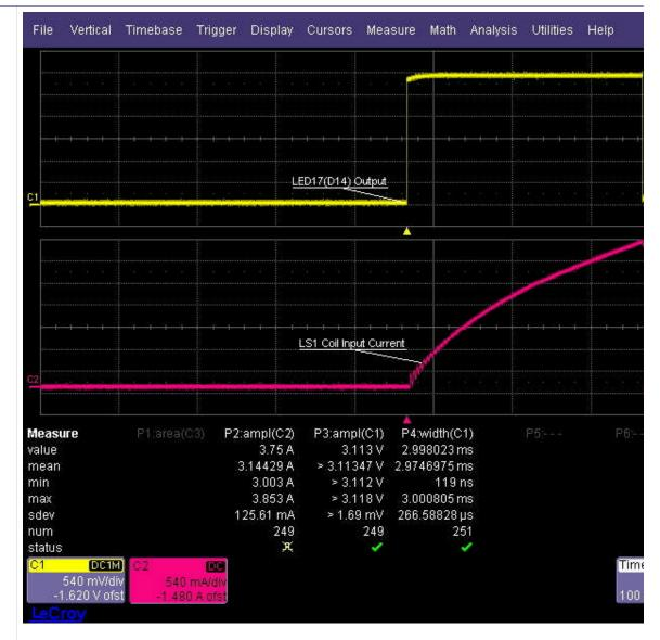
So from all this data, if you look at the mean amplitude for C1, you see that it is consisten means that the LS1 coils can fire at that voltage. The mean pulsewidth of C1 is always abc program into MS. This must be a firmware bug, I will post this on msefi.com.
